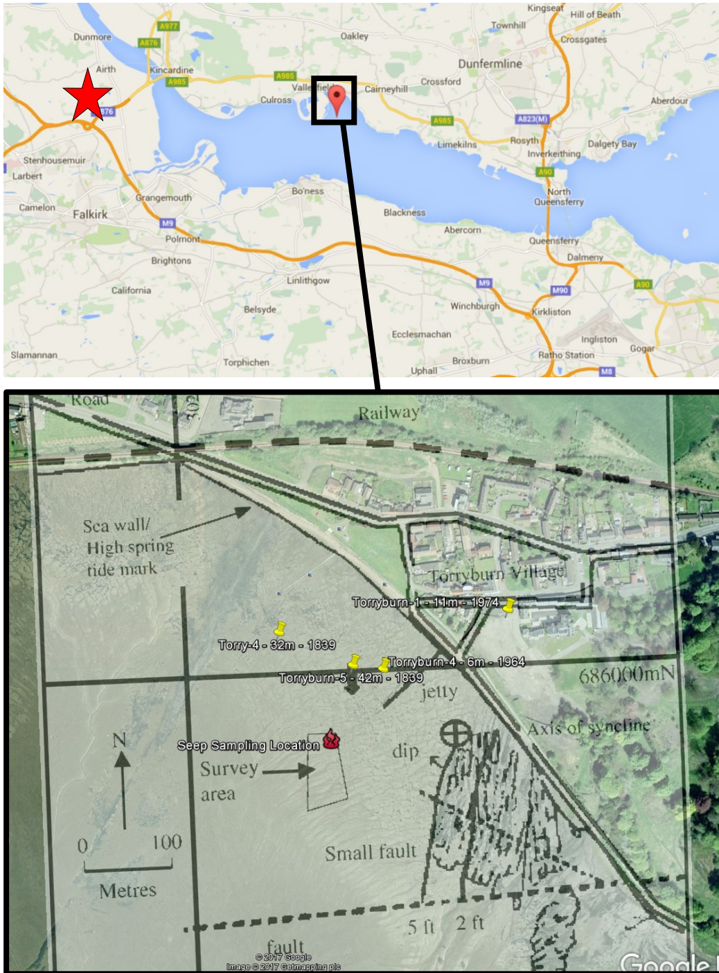
Figure 5-3 – Maps of Torry Bay. UPPER: Location map of the Firth of Forth with the Airth field (red star) and Torry Bay area (black box). LOWER: Expanded Torry Bay area with map overlay adapted from Judd et al. , (2002). Seep area can be seen in the “survey area” box. Actual sample location is indicated by the red flame. Yellow pins represent a selection of nearby deep well borings for coal exploration, denoted by Name-depth(m)-year drilled.
