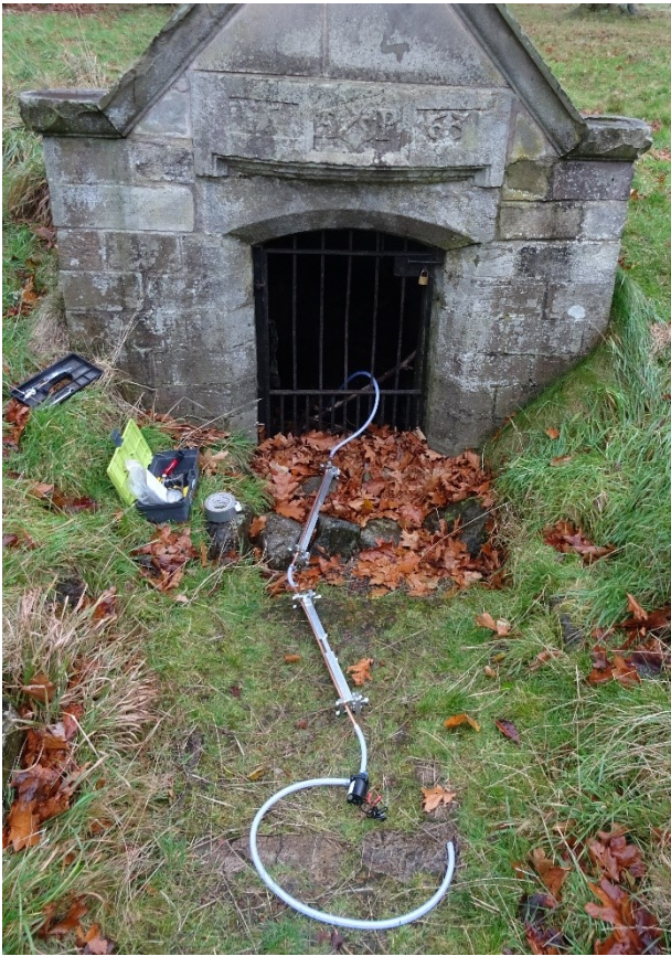
Sampling of St. Catherine's well waters. Copper tubing and battery-driven pump on the outflow side can be observed.
