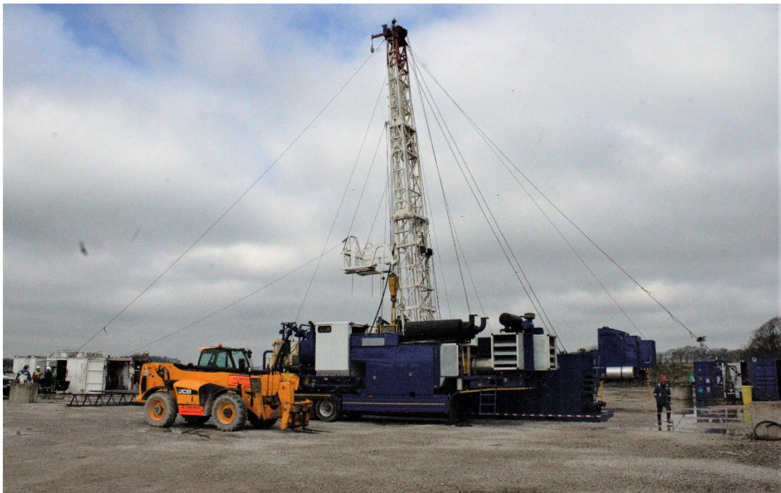
Figure 5-5 – Photograph of the workover rig at Cuadrilla's Preese Hall shale gas site. Gas sampling was undertaken while a cement packer was being drilled out as part of remedial operations.
