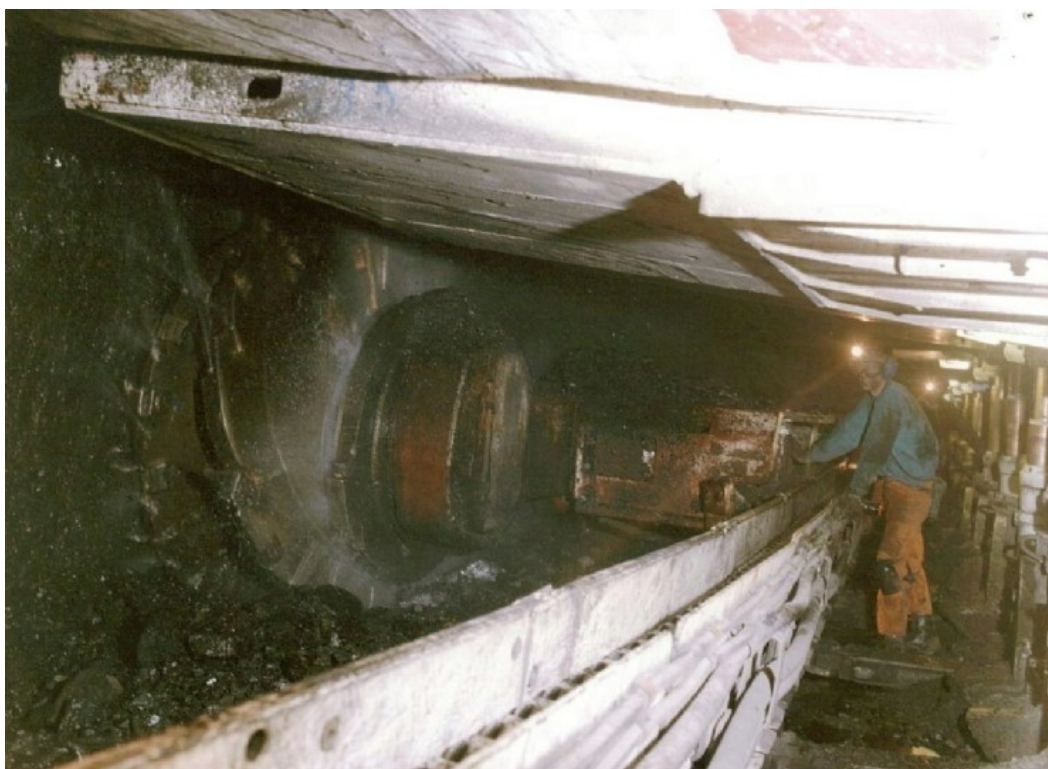
Shearer cutting the Top Hard seam at Bevercotes, circa ~1990's. © forum user "Bones"; https://www.aditnow.co.uk/ and reproduced here with kind permission.
