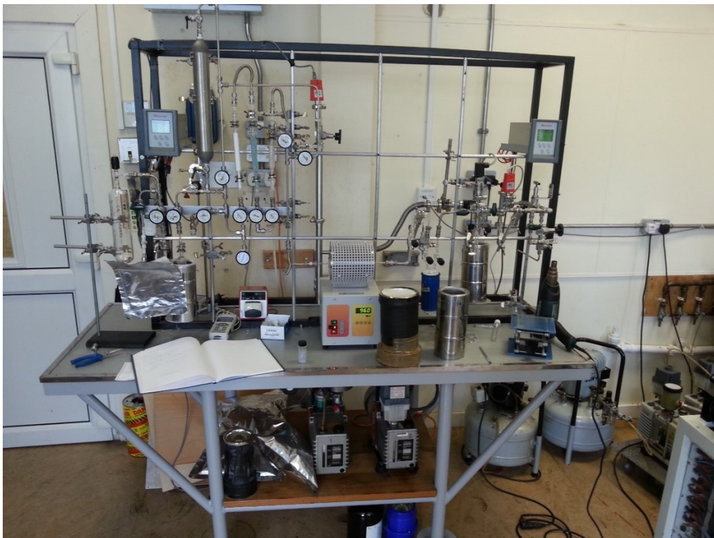
Figure 2-6 - Gas combustion line at SUERC, East Kilbride, for stable isotope analysis.
