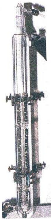
Figure 3.5 Bubble column for measuring Henry's law coefficients
