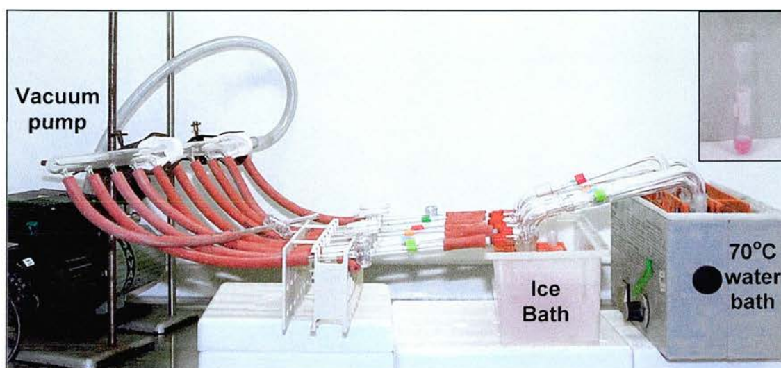
Figure 2.1. Vacuum distillation equipment used for measurement of LOX enzyme activity. When the vacuum pump is switched on samples in the 70°C water bath boil under vacuum and pass along the swan-neck tubes to condense in the ice bath. Insert shows assay tube with assay medium below a Kleenex tissue inserted to prevent rapid evaporation.
