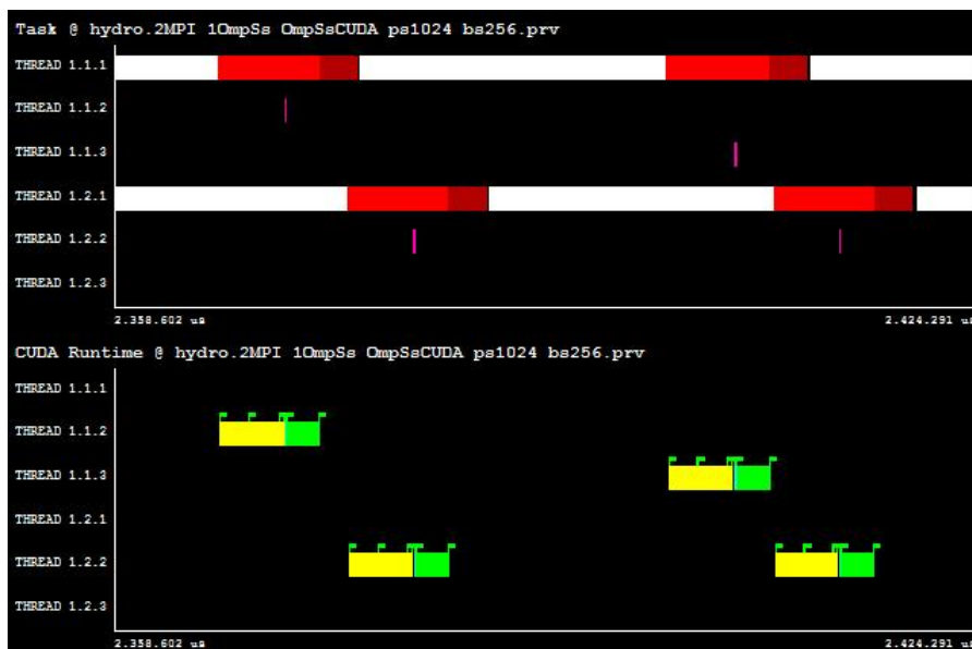
Figure 8: Zoom of Figure 7 showing a pair of GPU tasks instantiated by each process (top) and CUDA runtime calls by the Nanos++ runtime to transfer data from CPU to GPU (yellow) and in the reverse direction (green)
