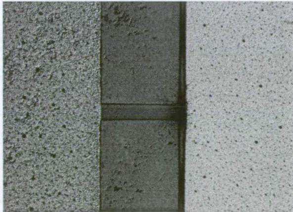
Figure B.7. Microscope picture in 200X magnification of 1\mu\text{m} thick Al electrodes after 160 minutes of etch in \text{NH}_4\text{F} : \text{CH}_3\text{COOH} . \text{NH}_4\text{F} : \text{CH}_3\text{COOH} clearly increases the etch selectivity between \text{SiO}_2 and Al and provides intact electrical contacts even after long release etches.
