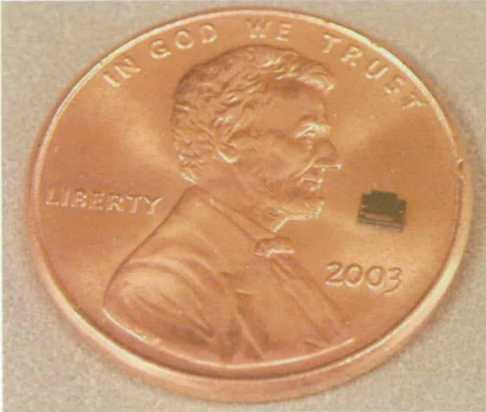
Figure 1.1. Micromachined on-chip resonator on top of an US one cent coin. In future, multiple micromachined resonators will be able to be interlinked to form mixers, filters and oscillators on one single chip, providing a reduction in cost and size and an increase in functionality in multi-band wireless transceivers. (Picture courtesy: Discera Microcommunication Technologies) [124].
