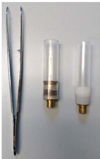
Figure 2.10: Holders used for the microCT analyses.
