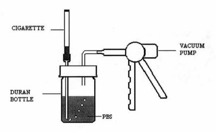
Figure 7.1 Apparatus used in the production of the water soluble components of cigarette smoke.
