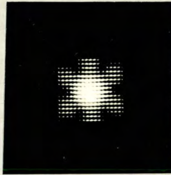
b) A pixelated filter in the Fourier transform plane
