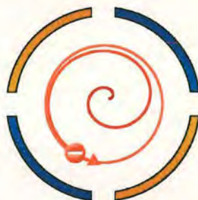
Figure 3-27 A depiction of ion cyclotron resonance. The ions are given kinetic energy by the electric field generated by the excitation plates (orange), and are made into a spatially coherent ion packet. As the ions pass the detector plates (blue) a current is induced, which can be transformed into a time domain ion signal. Diagram adapted from Reference 71.
