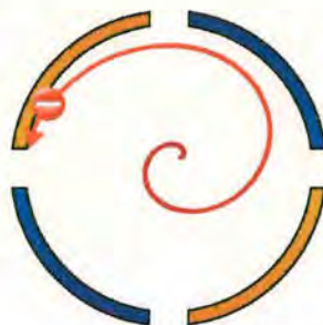
Figure 3-28 Ions of a given mass-to-charge value, and hence cyclotron frequency are given an excess of kinetic energy by the exciting electric field such that they are given a cyclotron radius in excess of the ICR cell radius, and are lost from the cell. Diagram adapted from Reference 71.
