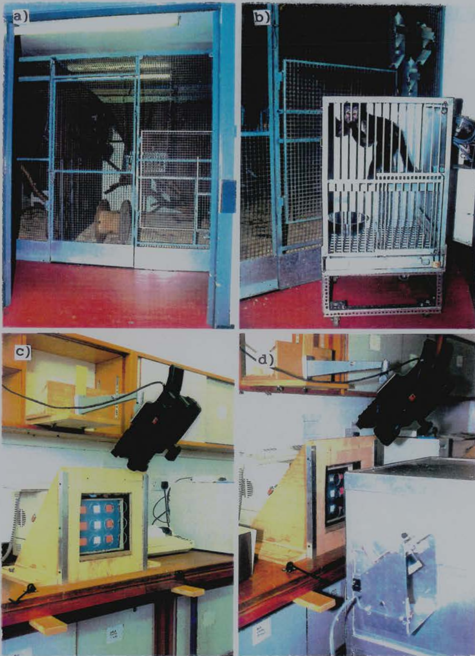
Fig. 4.1 The experimental set up used for this and the following experiments. a) The indoor cage where the colony of capuchins is housed. b) The monkey spontaneously enters the individual testing cage. c) The testing station provided with touch sensitive computer monitor and video camera. d) The cage with the monkey is hooked in front of the monitor (on the side of the cage, the food dispenser can be observed).
