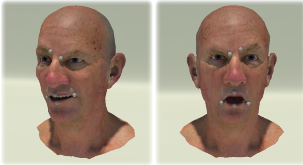
Figure 3.10: Application to facial model in a FacelK fashion. The user moves the control points and the rig parameters of the face are computed to satisfy the constraints.
