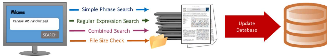
Figure 5.7 Four main workflows that use four different functions initially, and then share the same update database function
