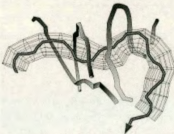
Figure 2.14: Diagram illustrating the tube model for the reptation of polymers. Other polymer in solution act as obstacles, and are represented by the tube as indicated. (Reproduced from [40]).
