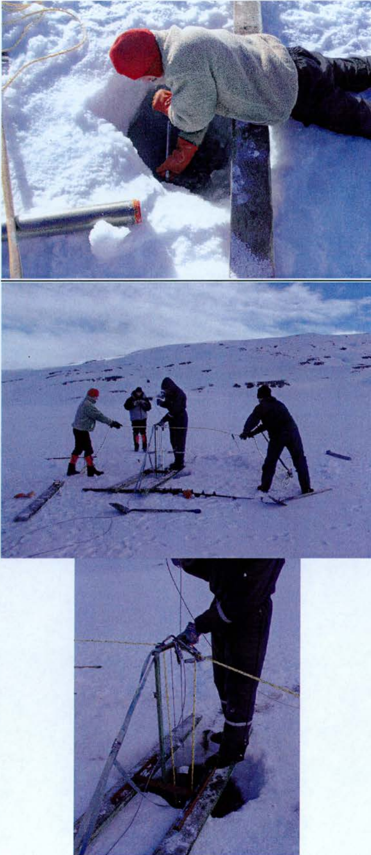
Figure 2.20: Winter coring on Hofsvötn. (Top) Drilling through the ice. The ice drill is 2m long from handle to tip, and Jökull is demonstrating the total thickness of ice and overlying snow/slush! (middle) Piston coring: Skúli and Jökull are raising and lowering a weight to hammer the core tube into the
