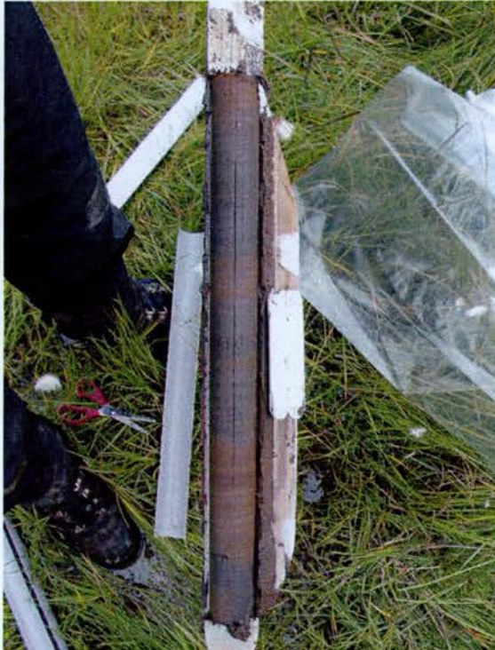
Figure 2.19: An example of a core sample extracted with Russian corer. This particular sample was not used (taken near the lake margin), but shown as the camera was not risked on the lake coring platform!
