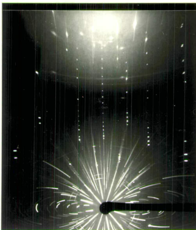
Fig. 4.6 X-ray reflection diffraction photograph of CdS on mica (Knudsen source).
