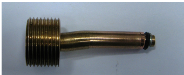
Figure 6.24: An example of a mechanical failure of the pressure cell setup. The piston was buckled on the pressure increase at around 10 kbar.
