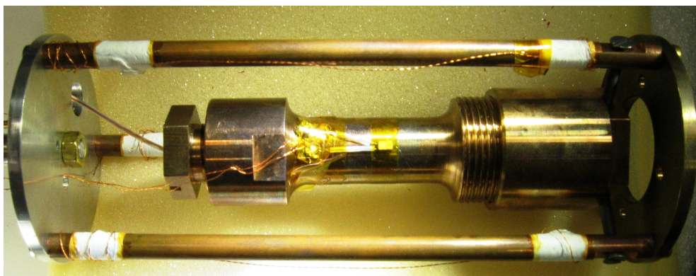
Figure 6.5: The piston cylinder cell mounted on the cryostat probe. The thermometer was attached as close as possible to the sample location on the side of the cell.
