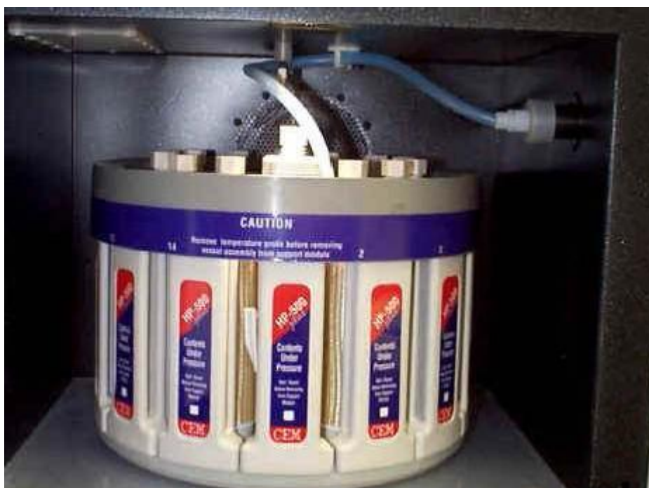
Figure 2.14: Schematic of microwave running system (carousel, closed system vessels, blue pressure sensor tube)
