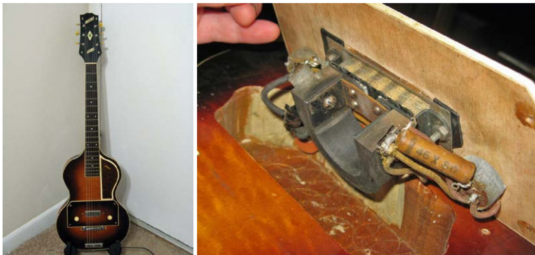
Figure 10.7 – Slingerland “Songster” model 401 electric Spanish-style guitar and its massive six-coil pickup, late 1930s.
