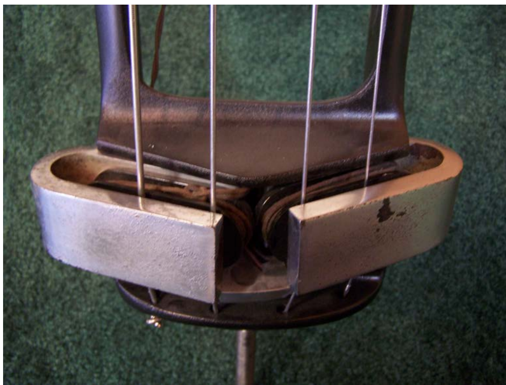
Figure 6.2 – The horseshoe pickup of the Electro Bass Viol (cast metal version with black crinkled finish).
