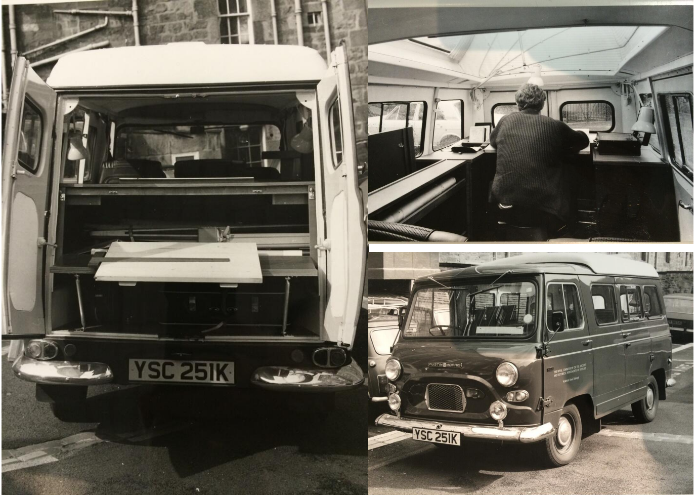
Figure 7.5: The Commission's Austin Morris J4 that replaced the Commer Van in 1972. Like the Commer, the J4 was specially outfitted with everything the Commission's staff might need in the field when undertaking surveys. Vehicles like the J4 became an integral part of the Commission's practice in the field. They were a mobile office that transported staff and the Commission, throughout Scotland. Source: photograph author's own from Royal Commission on the Ancient and Historical Monuments of Scotland uncatalogued material.
