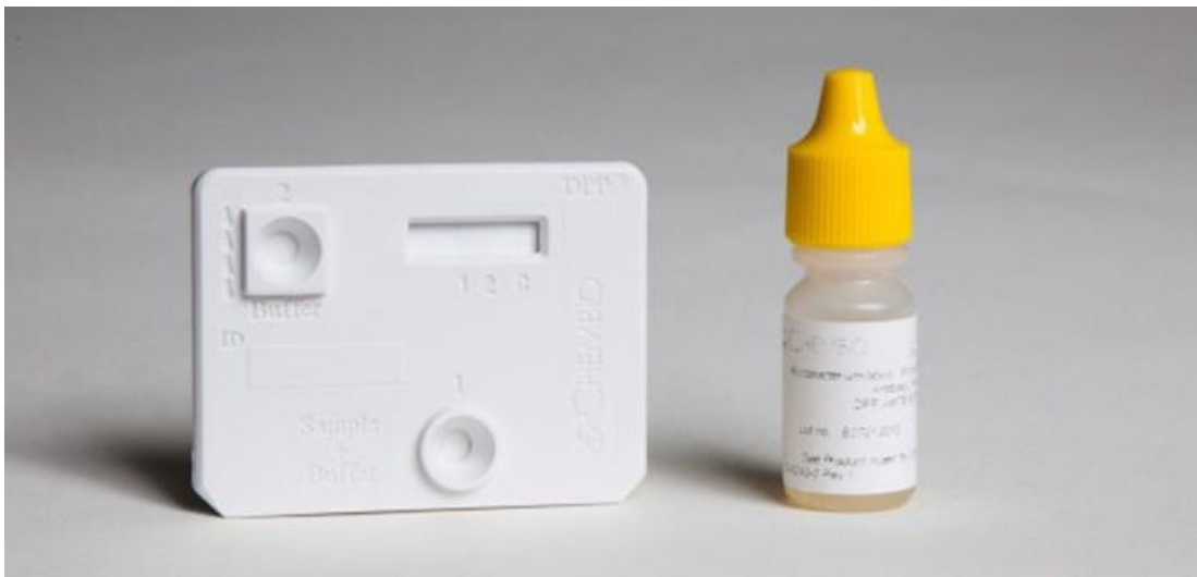
Figure 1.14: The VetTB Assay for Cervids. The sample well (top left) and the buffer well (bottom centre) form a ‘T-shape’ nitrocellulose strip. A positive antibody response leads to the development of a visible line within the result window (top right) after approximately 20 minutes incubation at room temperature.
