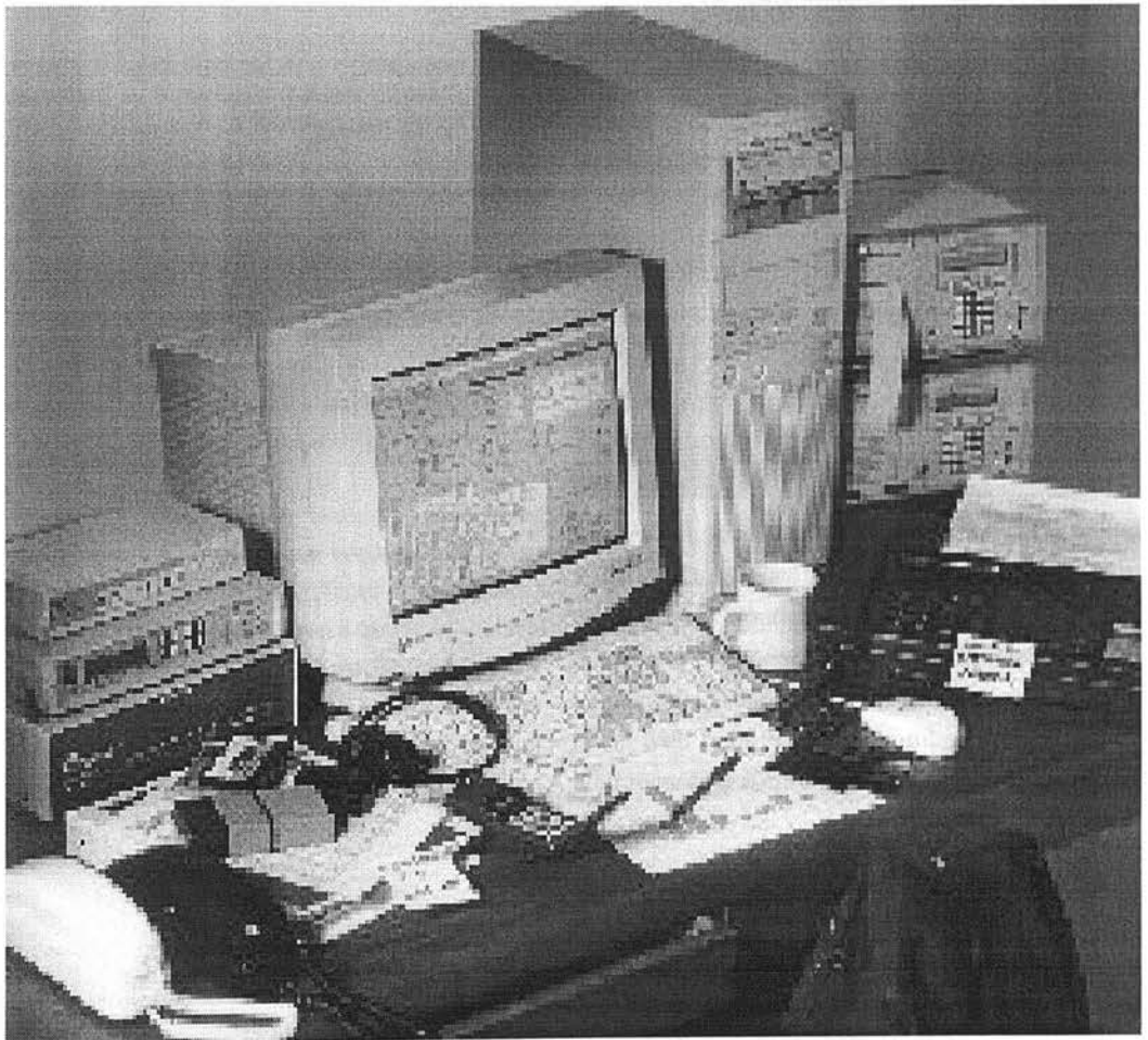
Figure 6.1.1b: A number of DNRs are seen here connected with a designated computer. The marriage between DNRs and especially designed digital software allows the synchronous analysis of electronic call detail records, phone company toll record files, and cellular call records.
