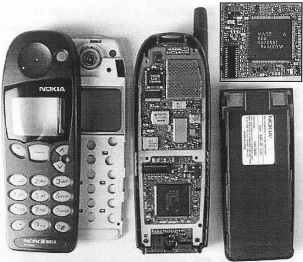
Figure 6.2.3 The interior of a cellular phone handset contains a sophisticated computer system. The CODECs, which convert sound signals to binary signals and vice-versa, are contained within the microprocessor. The microprocessor is the large square located at the bottom half of the inside panel –see insert (source Nokia Ltd.).
