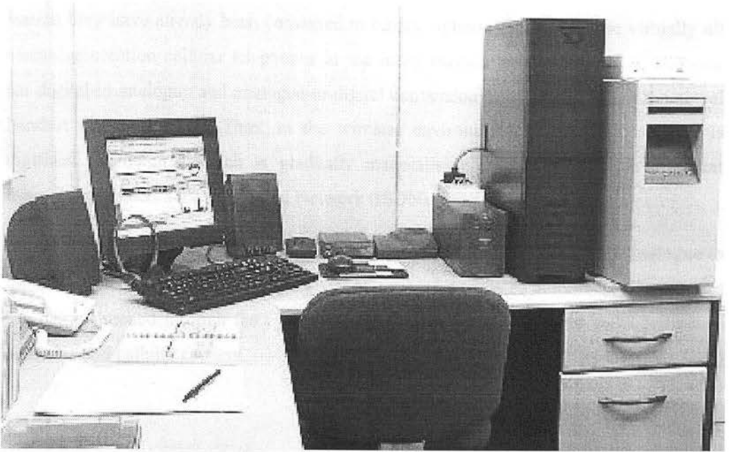
Figure 6.3.1a: The above picture shows a state-of-the-art digital collection unit. The large white box on the right is a Magneto Optical jukebox, a content-storage appliance that records and stores intercepted telephone content data. Storage appliances such as these can hold up to 16 removable discs, each with a storage capacity of 180 hours of uncompressed audio. The large black box next to it is a collection server, which receives intercepted call data and content (original photograph).
