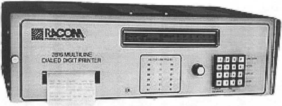
Figure 6.1.1a: This particular DNR, known as Racom 2816D DNR, is used exclusively by government and law enforcement agencies in the US, UK and other countries. It can simultaneously monitor all call activity on up to six target lines. For each intercepted call, Racom 2816D displays and prints a detailed call record (source: Racom Ltd.).
