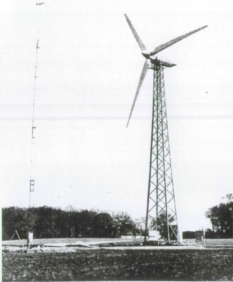
Figure 4.2.2(i) Vestas V20/100 wind turbine at the Test Station for Windmills, Risø, Denmark.
