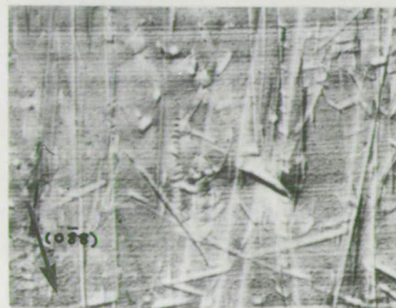
[112] [111] Transmission topographs of helical dislocations. Lang Ag K \alpha 1 mm
