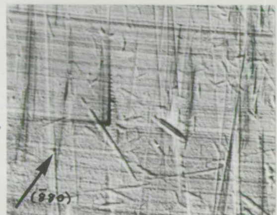
[112] [111] Transmission topographs of helical dislocations. Lang Ag K \alpha 1 mm
