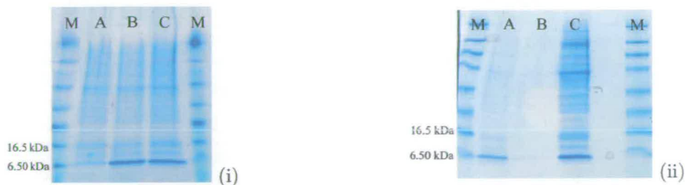
Figure 6.1: SDS-PAGE showing the results of the test of the dilution method for the SP-Sepharose gravity flow column. For (i), 300 \mu\text{l} of each sample was TCA precipitated for the gel. Samples A and B did not contain SP-Sepharose beads from their samples as the beads had been spin-out. Therefore only the surrounding buffer, and any protein not stuck to the beads, was loaded onto these lanes. For gel (ii), 15 \mu\text{l} of SP-Sepharose beads from both samples A and B were washed in their respective dilution buffers to ensure only protein that had stuck to the SP-Sepharose beads would be present on the gel. Again, 300 \mu\text{l} of Sample C was TCA precipitated for this gel. On both gels (i) and (ii), the samples on the gel are marked as follows: (M) Marker; (A) sample A; (B) sample B; (C) sample C. The protein molecular weight marker used was the New England Biolabs Broad Range Prestained Protein Marker P7708G
