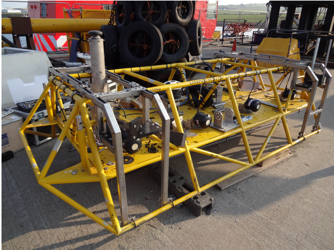
Figure 3.6: Top instrument frame being prepared for turbine deployment 5. The starboard SBDPs are visible mounted along the near edge with the AWAC behind in the centre. The outriggers for the focus beam SBDPs have been installed but the sensors themselves are not yet mounted.
