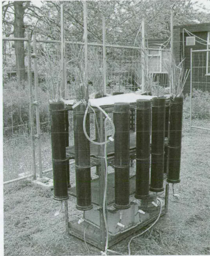
Figure 3-1. Constructed wetland filters (May, 2004)
