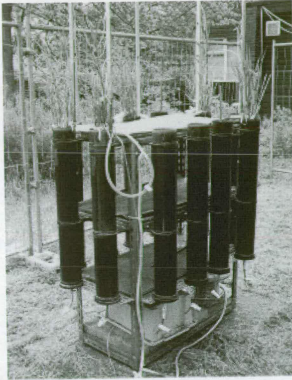
Figure 1. Constructed treatment wetland rig (The King's Buildings campus; The University of Edinburgh) in May 2004.
