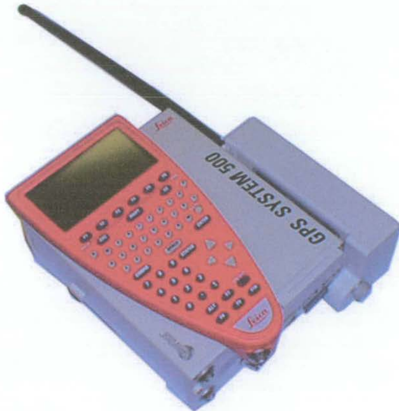
Figure 4.4 Photograph of the GPS System series 500 receiver, terminal (keypad) and radio modem (right, with aerial) (from Geophysical Equipment Facility: Natural Environment Research Council (NERC), 2004)
