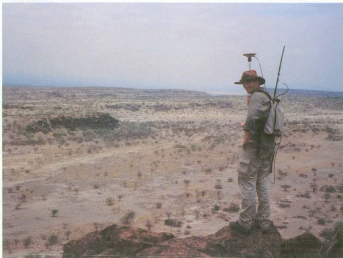
Figure 4.5 Photograph showing the main GPS rover assembly: an antenna mounted on a 2m pole and a receiver/radio modem stowed in a rucksack. The black aerial protruding from the top of the rucksack is for receiving the radio data-link from the reference antenna. In the background of the photo are the faults of the Ilainymok region, described further in section 4.5.
