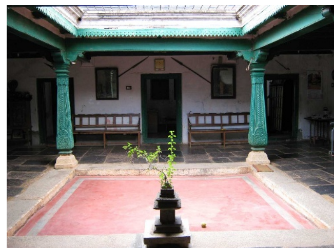
Figure 10. Old interior. This view shows the multipurpose area with locally available material. It reflects the maximum use of daylight and the least furniture resulting in very low operational costs
