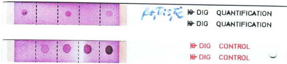
Plate 5.11 Experiment 9 : Example of quantification of labelling efficiency for \beta -tubulin, Tri5 and Tri6 DIG-labelled probes using test strips. The control teststrips coated with positively charged nylon membrane, are loaded with DIG labelled control DNA in the quantities 3, 10, 30, 100 and 300 pg.
