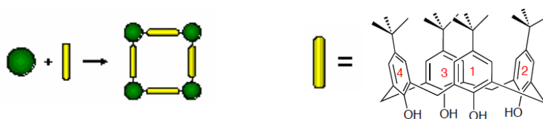
Figure 3-1: Schematic figure of metal-organic frameworks with metal clusters and linkers. The structure of calix[4]arene which is a potential linker is shown on the right.
