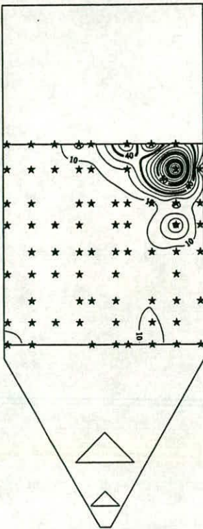
Fig. 5.19c BG0302: Mean velocity: Vertical diametral section C-G: Contours and spot values
