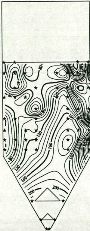
Fig. 5.14d BG0302: Remaining mass: Vertical diametral section D-H: Contours and spot values
