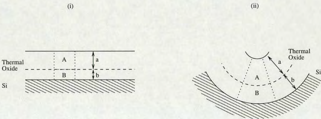
Figure C.1: The variation of oxide/silicon thickness with topography. (i) The ratio (b/(a+b)) of the thickness of the silicon consumed to the thickness of the oxide grown is given by the ratio of the volumes (B/(A+B)) , and hence the ratio of the molar volumes of Si and \text{SiO}_2 (0.44). (ii) The ratio of the thicknesses (b/(a+b)) is not directly proportional to the ratio of the volumes (B/(A+B)) and hence b/(a+b) < 0.44 .
