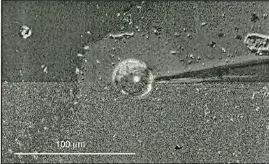
Fig. 3: Manoeuvring an isolated snail neuron onto the patch aperture. Scale bar = 100 \mu\text{m} . The soma diameter is approximately 35 \mu\text{m} . Transmission microscopy allows the backside cavity walls (85- \mu\text{m} square) to be dimly lit; the aperture is indicated by the bright light shining from underneath the device.
