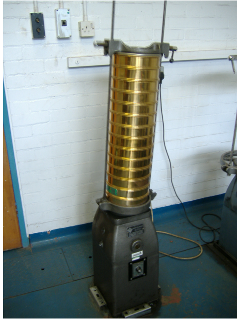
Figure 7.10. The sieves used to determine the particles size distribution.
