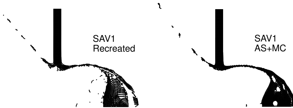
Figure 4.34: Particle positions of the high-velocity impact problem 8 \mu\text{s} after impact. The results are for the recreated SAV1 scheme from Mehra and Chaturvedi [141] and SAV1 combined with artificial stress (AS) and the adapted mixed correction (MC).
