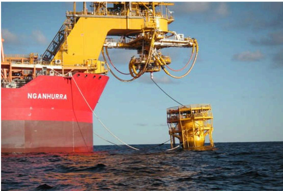
**Figure K. Disconnectable external turret mooring. Source: Smith (2009)**
