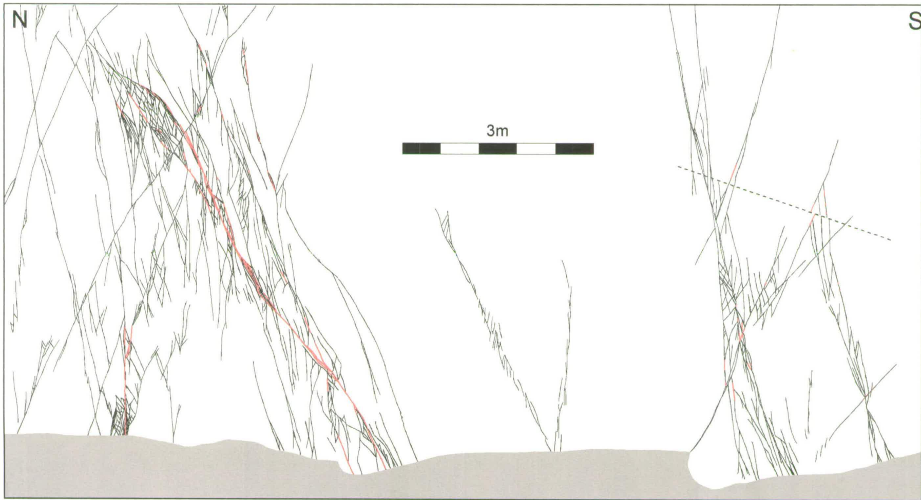
Figure 4.11. Detailed sketch of structures in the Cement Bridge footwall block (face dipping 40\text{-}80^\circ to the west). Black lines are deformation bands, and red lines are slip-surfaces. Grey fill is sand at the base of the outcrop. The dotted line on the right-hand side of the diagram is a bedding surface along which the deformation bands have been offset.
