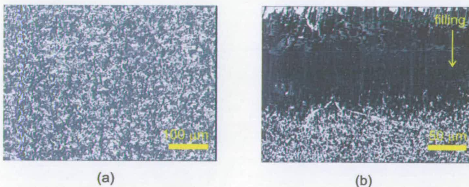
Figure 5.28: Micrographs showing the difference in texture between the central area of the cell (a) and region adjacent to the filling edge (b) observed in cells filled with the FLC+PVCi mixture. The textures were obtained just by cooling slowly to room temperature after filling without exposure to LPUV light.
