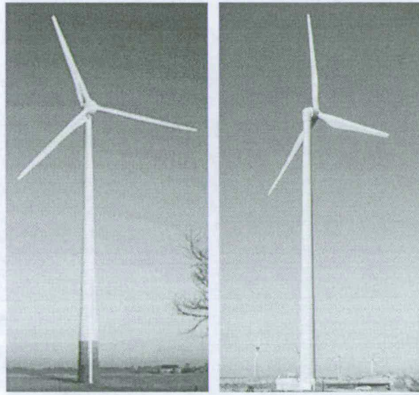
Figure 4.1. Enercon E-88 2MW wound rotor direct-drive wind turbine ( left ) and Harakosan Z-72 2MW permanent magnet direct-drive wind turbine ( right ).
