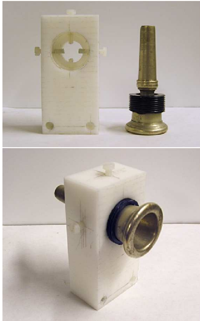
Figure 6.10: New mouthpiece holder; showing removable central section and stabilising screws.
