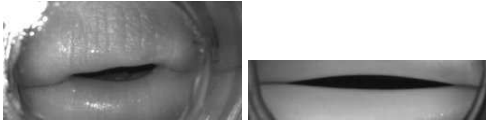
Figure 4.21: Maximum width of the opening of the lips of ( left ) player TJ playing the note Bb_2 at mf and ( right ) the artificial mouth playing note E_3 at 97dB
