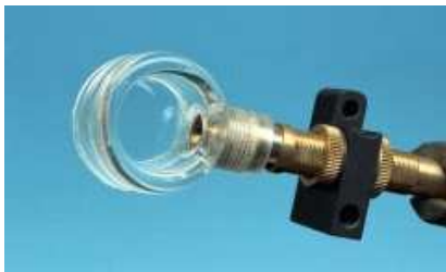
Figure 4.1: Transparent mouthpiece for trombone
