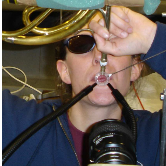
Figure 5.2: Photograph of the experimental equipment used for measuring the motion of a horn player's lips.
