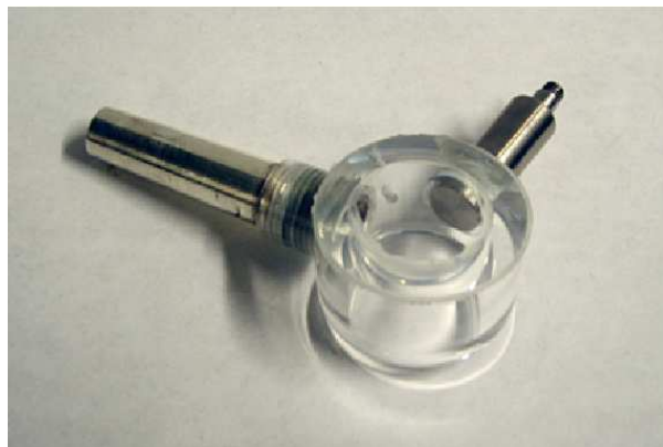
Figure 4.41: Transparent mouthpiece with PCB microphone.
