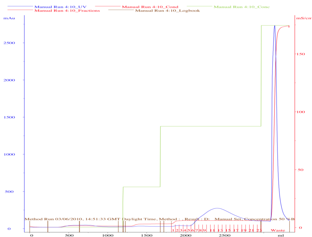
Figure 3.6: Anion exchange chromatography purification of the MSP-1 hybrid. Conductivity (red line), elution buffer percentage (green line), and protein concentration as measured by absorbance at 280 nm (blue line). Red numbers on the X-axis represent the fraction number of 50 mL eluted fractions from the CptoQ anion exchange column. MSP-1 hybrid absorbs UV light poorly due to its low extinction coefficient, and thus peak elution height is correspondingly low.
