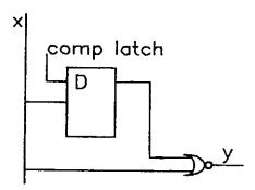
Figure 2.12: the fault tolerance logic
