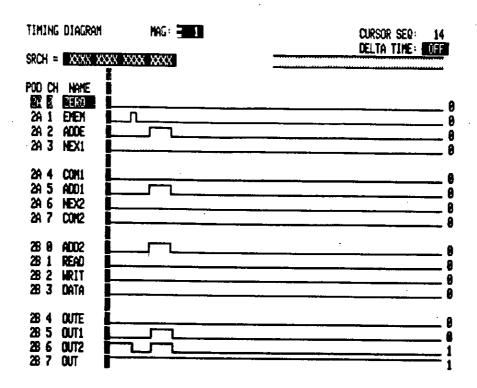
Figure 3.1: The emem signal initializes the chip by setting all of the tags in the empty tag group and by establishing the correct internal state. Note that the invalid out2 setting is corrected.
