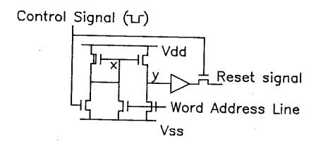
Figure 2.6: the non-cascading unit
