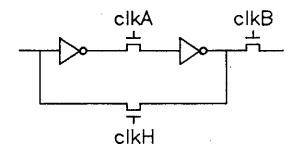
Figure 2.2: a semi-static shift register bit cell
