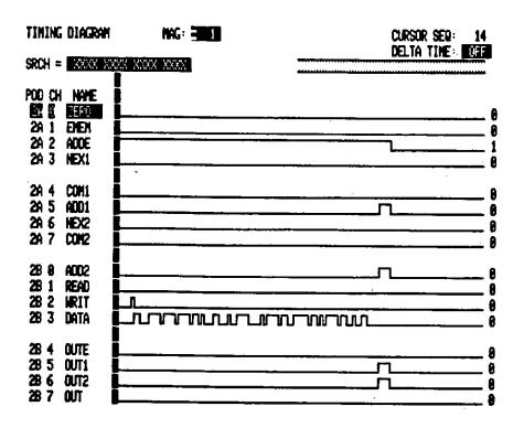
Figure 3.2: By addressing the empty tag group and initiating a write operation, a data word may be entered into memory.
