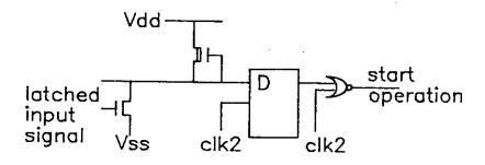
Figure 2.8: the start operation signal
