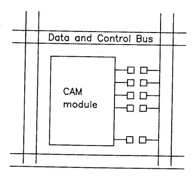
Figure 2.16: a discretionary wiring scheme
