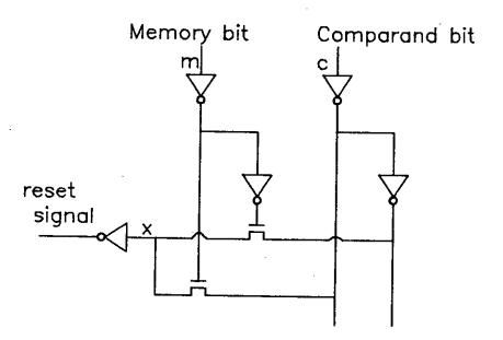
Figure 2.4: the comparison logic
