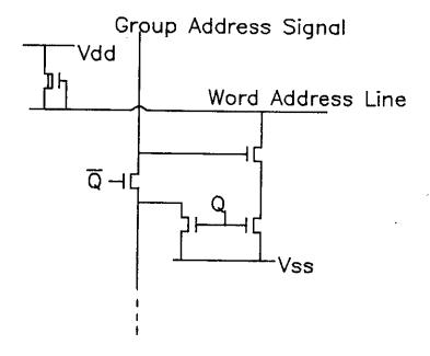
Figure 2.5: the addressing logic
