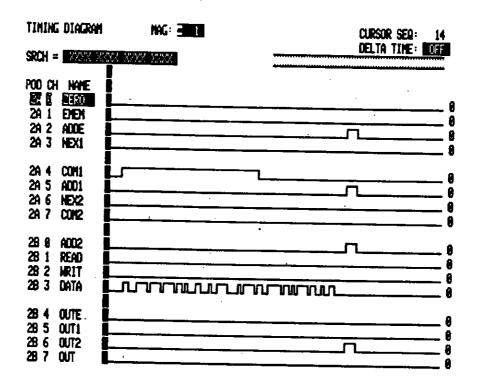
Figure 3.3: The same data work is used in a masked comparison, on tag group 1, and a successful matching is indicated by the fact that out! no longer follows add!.
