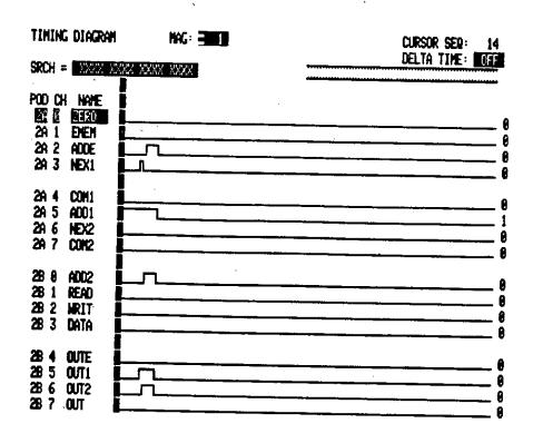
Figure 3.5: The comparison tag is reset by a next command ...
