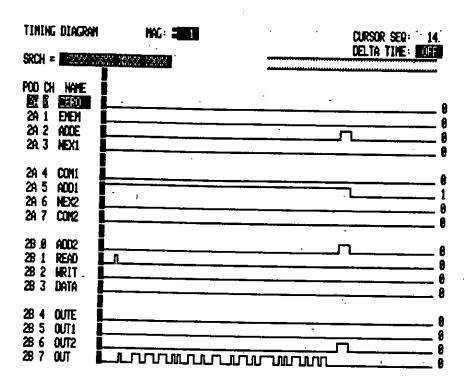
Figure 3.4: The matching word in memory is output by addressing comparison group 1 and initiating the read operation.
