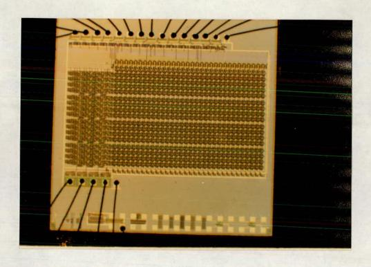
Plate 1: the basic component: 16 words of 64 bits, 4.53 x 3.65mm in a 5 x 5mm frame.
