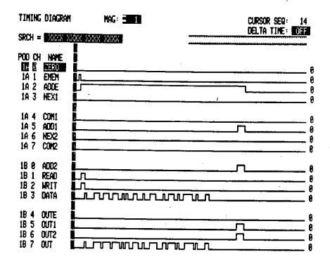
Figure 3.8: This display shows the signals associated with the initial elimination test pattern.
