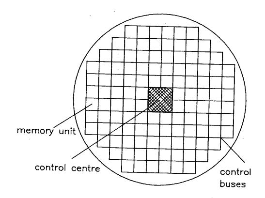
Figure 2.15: the signal distribution logic
