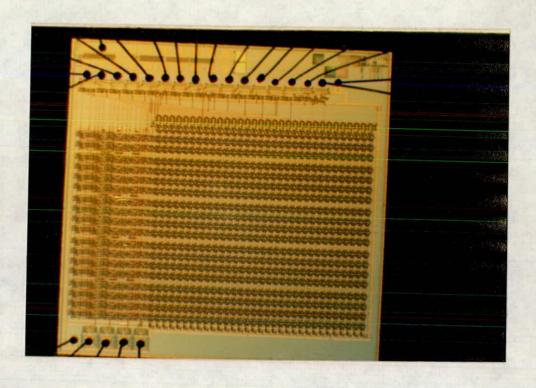
Plate 2: the enhanced component: 18 words of 64 bits, 4.72 x 4.35mm in a 5 x 5mm frame.
