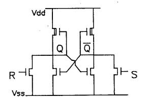
Figure 2.3: the latch realization of a tag
