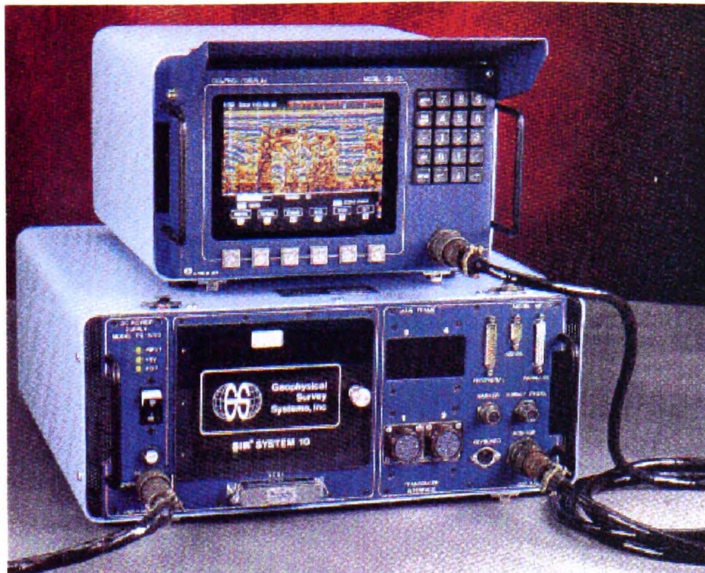
FIG. B.2 GSSI Digital Radar System SIR 10: control unit and display.
