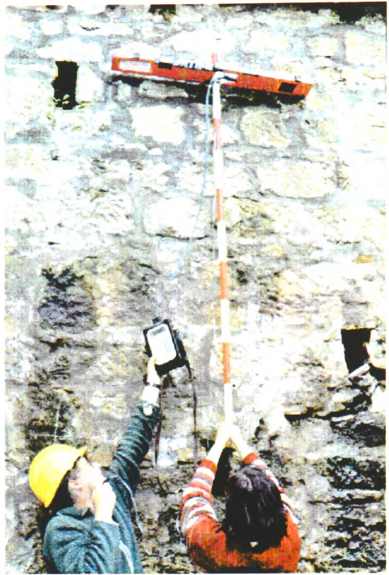
Fig. 5.14-In situ conductivity data collection: a)instrument lifting positions, b) in contact.
