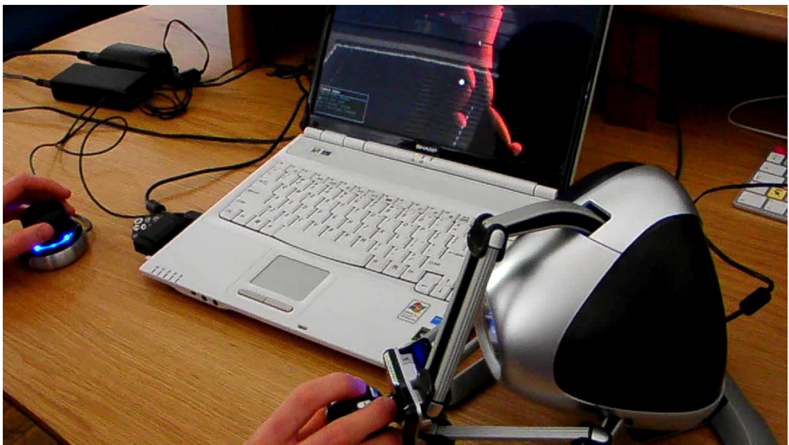
Figure 3.28: One of the animators working in the haptic workspace using the Falcon haptic device
