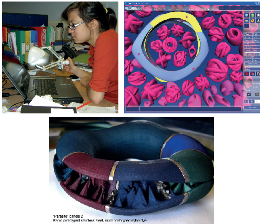
Figure 1.5: Bandoorkwala working with the haptic device, a screenshot of the application with the designed digital artifact and a 3-D printed bracelet. Images courtesy of Anarkik3D
