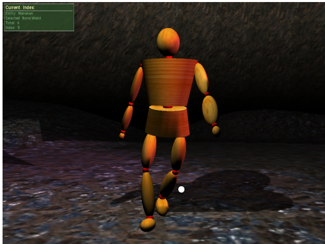
Figure 2. The 3-D virtual space. The white sphere is the visual representation of the haptic device
