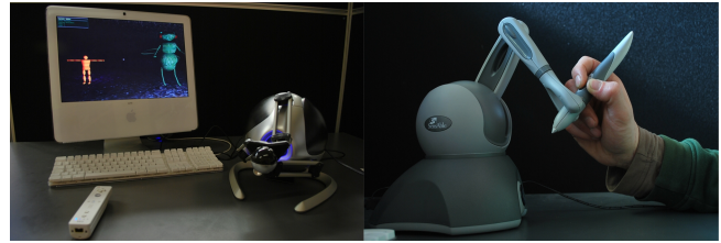
Figure 3. The setup with Novint Falcon and the Wii Remote (left) and the Sensable Omni™ (right)
