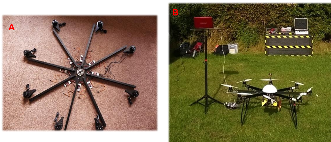
Figure 3-17: (A) Main propulsion components of the UAS before assembly; (B) The completely assembled UAS carrying a dummy payload to simulate the gimbal and sensor package weight.
