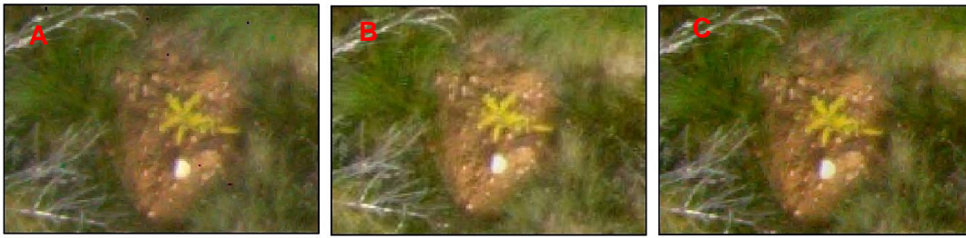
Figure 3-21: Example image of a conifer sapling; (A) the converted RAW image showing bad pixels (black and coloured speckles across the scene); (B) JPEG image with no bad pixel visible; (C) the converted RAW image after processing with CHDKPTP to fix the bad pixels (none can be seen).
