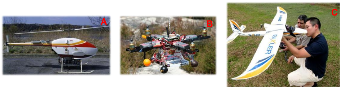
Figure 1-2: Example UAS of the three main types of UAS that have been used for remote sensing over the last decade; (A) a helicopter UAS (RPH2; Subaru, Tokyo, Japan) used to study riverbeds (Nagai et al. , 2007); (B) A multi-rotor UAS (custom built) used to study heathlands (Gademer et al. 2010; (C) A fixed wing UAS (custom built) used to study tropical wildlife (Koh & Wich, 2012).
