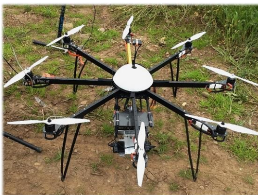
Figure 3-18: The completed UAS with sensor package attached and connected to the autopilot.
