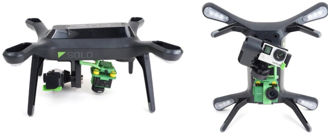
Figure 3-13: Side and underside views of a 3DR Solo UAS fitted with 3 axes brushless gimbal with GoPro camera attached, and a tilted fixed mount with MAPIR camera attached (green camera; MAPIR, 2018).
