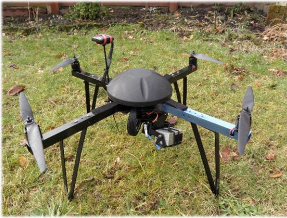
Figure 3-15: The quadcopter equipped with GoPro camera in small servo gimbal.
