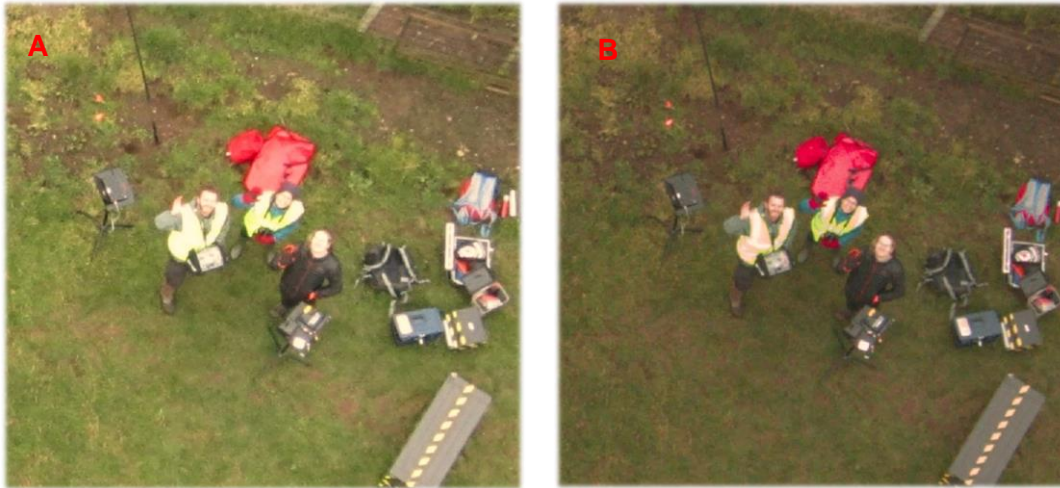
Figure 3-25: Example of a JPEG (A) and TIFF (B) image interpolated from the RAW file. More image noise and over exposure of bright objects can be seen in (A); Highlight recovery shows far more detail in (B) and less noise, but some brighter features get a pinkish tint (e.g. the fluorescent jackets).
