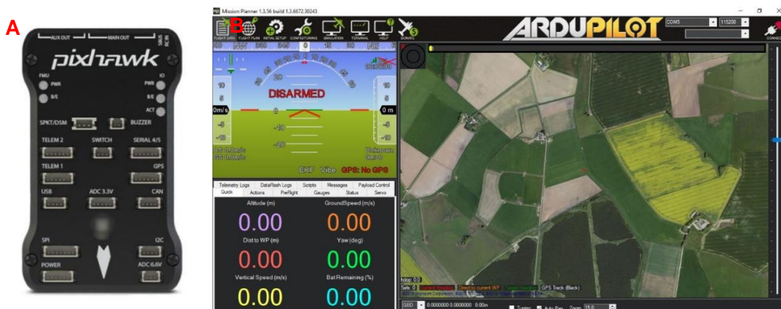
Figure 3-16: (A) 3DR Pixhawk autopilot (3DR, 2018); (B) Example of the mission planner GCS primary screen (indicates aircraft attitude via wireless telemetry).
