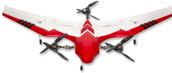
Figure 3-3: The FireFLY6 hybrid VTOL UAV (BirdsEyeView, 2018)
