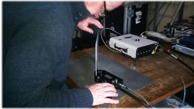
Figure 3-37: The SVC contact probe and spectrometer in use measuring a grey card target.
