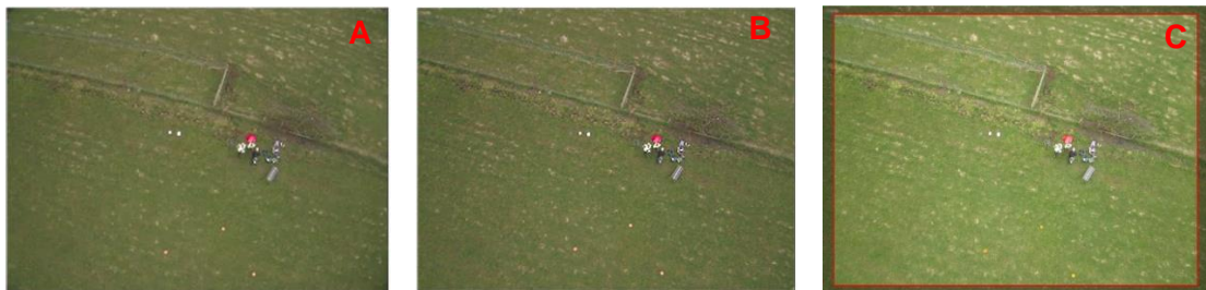
Figure 3-27: (A) An uncorrected TIFF image (note curve of fence line); (B) a corrected and cropped TIFF image; (C) a corrected and cropped TIFF image overlaid with its corresponding JPEG image to show extent of extra image footprint.
