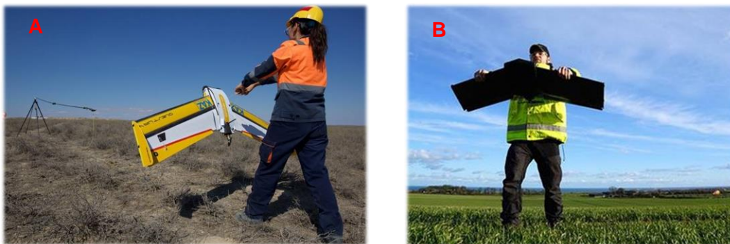
Figure 3-2: (A) A Quest Q200 being bungee launched (QuestUAV, 2018b); (B) A Quest Datahawk AG being hand launched (QuestUAV, 2018c).
