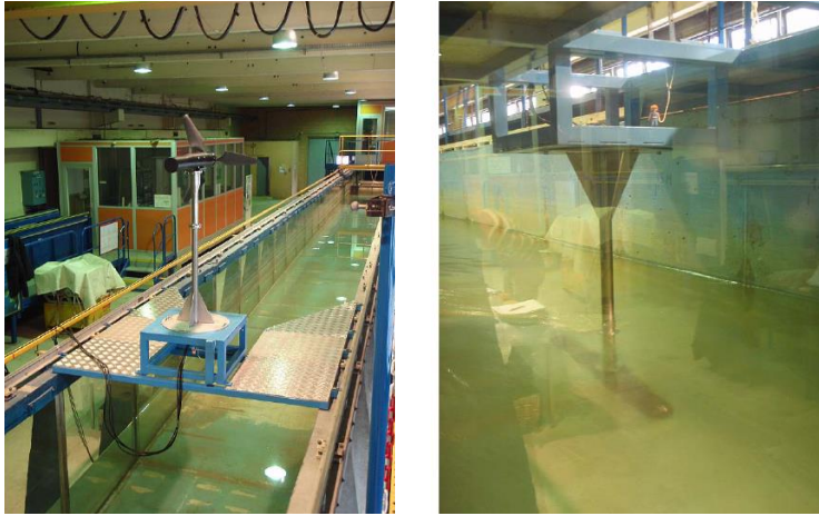
Figure 4.15: Case 3 images of the flume experimental set-up, with installed turbine and test rig, taken from Buvat and Martin (2010)
