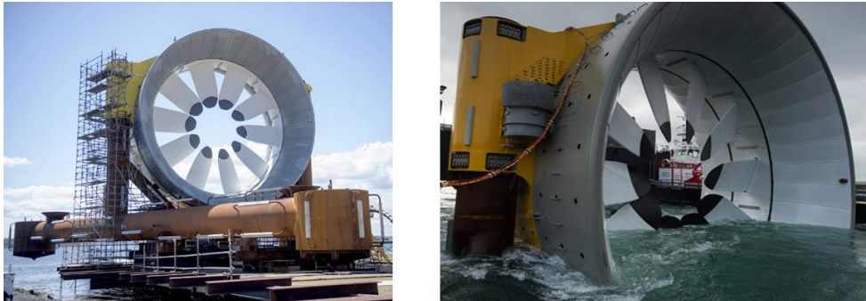
Figure 1.3: OpenHydro PS2: (left) 2 MW rated turbine for CapeSharp project, Nova Scotia; (right) 500 kW rated turbine undergoing installation at the Paimpol Brhat site, Northern France (images credit: Naval Group)
