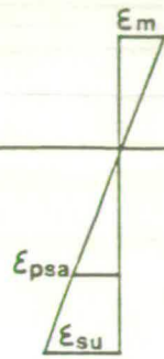
Fig. 8b Strain Distribution at Failure
