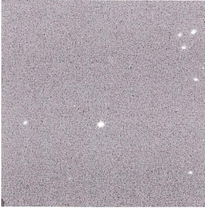
Figure 2.13: A reduced frame of PC 0025+0447 using the artefact-reduced flat field — scaling is linear in the range [\mu - 3\sigma (black), \mu + 3\sigma (white)], where \mu = 647 and \sigma = 0.0017\mu .
