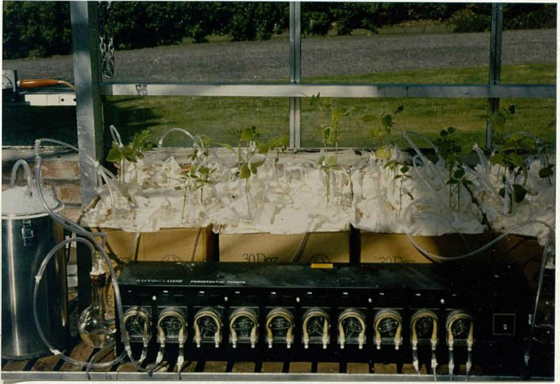
Plate 3.3 "Closed-vessel" system for comparisons of root growth in presence and absence of endogenous ethylene and carbon dioxide.
