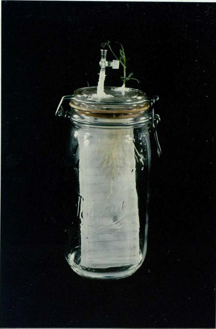
Plate 3.1 Root growth system using Kilner jar with perspex slope covered with filter paper "wick", based on system of Goodlass and Smith (1979).
