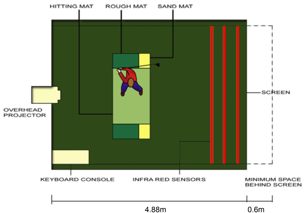
Figure 3.2. Plan layout of the simulator including infrared sensors and playing surfaces ( http://www.smartgolfeurope.com/html/spaceallocation.htm ).
