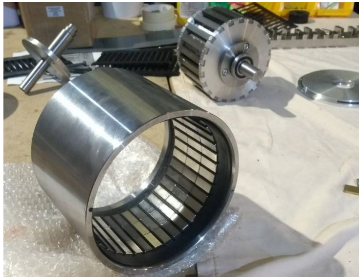
Figure 4.3: Gear outer magnetic ring
